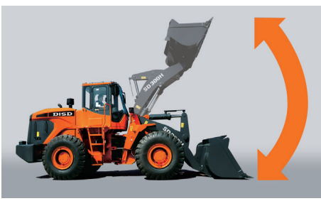
Arm Raise Kick-out and Return to dig function : reduce the intensity of your work and improve working efficiency.
