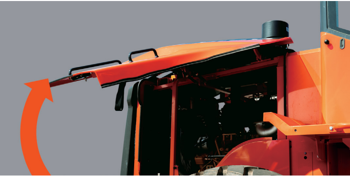
Full Tilting of Engine Cover With this one body engine cover, it is easy to repair engine and sub parts.
