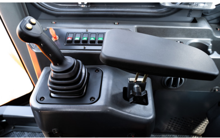
Pilot operating system provides comfortable machine control.
